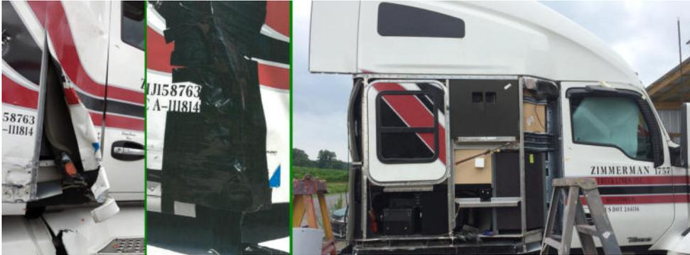
of safety was compromised.” Above you can see a collage of three photos: (Left) the damaged truck, (Center) the “tape job”, and (Right) the truck after repair (totaling over \$14,000 in damages) before the exterior panel was placed on. Our hats are off to Carol for keepin’ the wheels rollin’!
