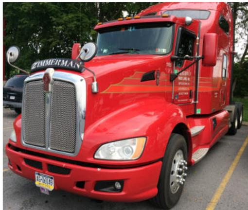
"Ten units will be for the Flatbed Division and five for the Van Division," Derek said. All will have Cummins 500 horsepower engines, driver-friendly Eaton "Endurant" 12-speed automated manual transmissions, 76" bunks, upgraded seats, refrigerators, and Kenworth's widely acclaimed Idle Monitoring System in place of the ThermoKing APUs now in use.
